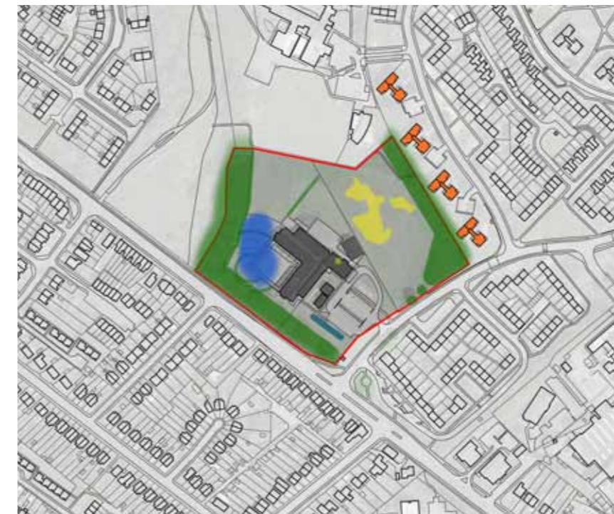
Site Boundaries, Flooding Risk and Pollution Scale 1:5000
